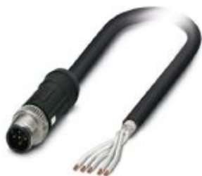
Sensor/actuator cable, 5-position, PE-X halogen-free, black, shielded, Plug straight M12 SPEEDCON, coding: A, on free cable end, cable length: 5 m, For railway applications
