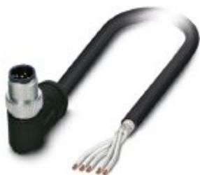
Sensor/actuator cable, 5-position, PE-X halogen-free, black, shielded, Plug angled M12 SPEEDCON, coding: A, on free cable end, cable length: 10 m, For railway applications
