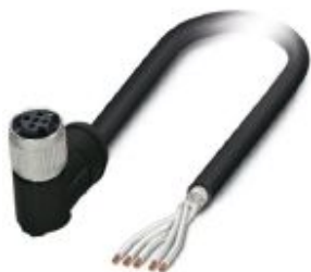
Sensor/actuator cable, 5-position, PE-X halogen-free, black, shielded, free cable end, on Socket angled M12 SPEEDCON, coding: A, cable length: 2 m, For railway applications
