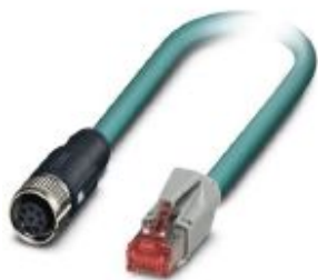
Network cable, Ethernet CAT5 (1 Gbps), 8-position, PUR, water blue RAL 5021, shielded, Plug straight RJ45 / IP20, on Socket straight M12 SPEEDCON / IP67, coding: A, cable length: 1 m
