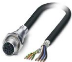
Hybrid flush-type socket, Ethernet, 8-pos., M12-SPEEDCON, rear/screw mounting with M16 thread, 360° shield connection with connected shielded hybrid cable
