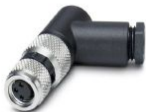
Connector, Universal, 3-position, Socket angled M8, Coding: A, Screw connection, knurl material: Nickel-plated brass, external cable diameter 3.5 mm ... 5 mm
