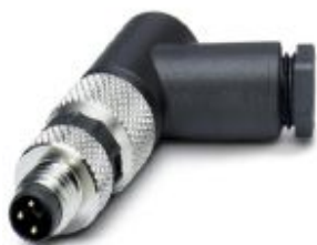
Connector, Universal, 3-position, Plug angled M8, Coding: A, Screw connection, knurl material: Nickel-plated brass, external cable diameter 3.5 mm ... 5 mm
