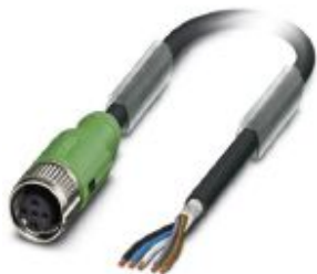
Sensor/actuator cable, 5-position, PUR halogen-free, black-gray RAL 7021, shielded, free cable end, on Socket straight M12 SPEEDCON, coding: A, cable length: 5 m
