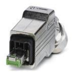
Push-pull connector (version 14), die-cast zinc, with RJ45 connector insert, 8-pos., with IDC fast connection technology, for 1 and 7-wire cores, 23 ... 22 AWG, for cable diameter of 5.5 mm ... 10 mm, cable outlet at the bottom
