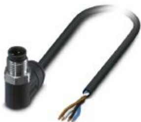
Sensor/actuator cable, 4-position, PE-X halogen-free, black-gray RAL 7021, Plug angled M12, coding: A, on free cable end, cable length: 5 m, for outdoor applications, with high-grade steel knurl
