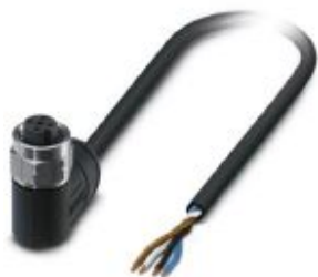
Sensor/actuator cable, 4-position, PE-X halogen-free, black-gray RAL 7021, free cable end, on Socket angled M12, coding: A, cable length: 2 m, for outdoor applications, with high-grade steel knurl
