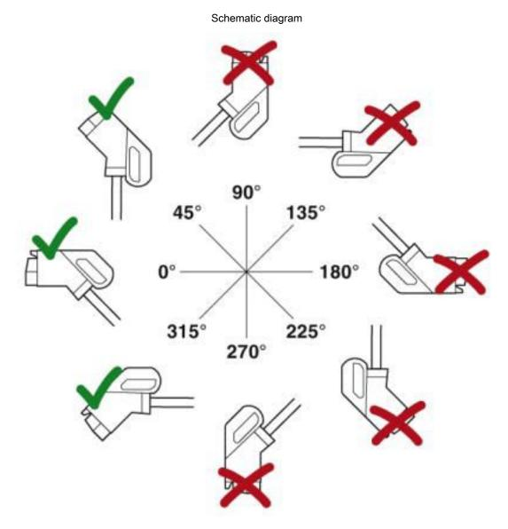
The resting position must be installed in the charging station such that the user cannot hang up the vehicle connector upside down ( $90^{\circ}$  to  $270^{\circ}$ ). However, positions rotated upward ( $45^{\circ}$ ) or downward ( $315^{\circ}$ ) are options for a resting position.
