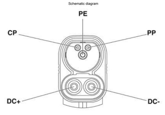
Pin assignment of the Vehicle Connector
