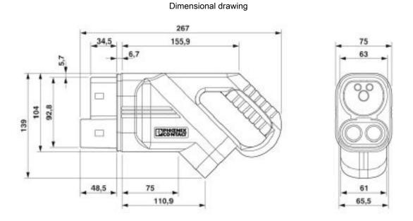
Ensure that the vehicle connector is placed in an appropriate resting position that ensures a minimum protection rating of IP24 in accordance with IEC 61851-1 for the entire time between charging. Use the dimensions of the vehicle connector to create this type of resting position. Detailed specifications can also be found in the download area.
