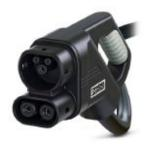
DC charging cable, with vehicle charging connector and open cable end, Housing color black-gray, For charging electric vehicles (EV) with direct current (DC), for installation at charging stations for electromobility (EVSE), CCS type 2, Combined Charging System, IEC 62196-3, 125 A / 1000 V (DC), D-Line 1.0, "PHOENIX CONTACT" logo, cable: 4.5 m, black, straight
