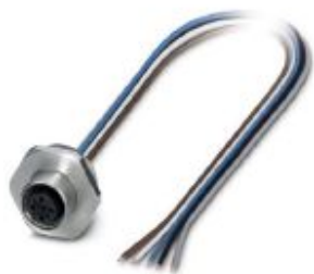
Sensor/actuator flush-type socket, 8-pos., M12, A-coded, front/screw mounting with M20 x 1.5 thread, with 0.5 m TPE litz wire, 8 x 0.25 mm 2 , brass version
