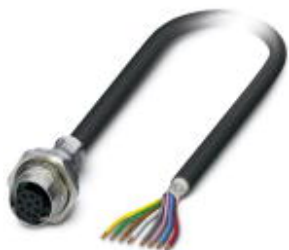
Flush-type socket, shielded, 8-pos., M12, A-coded, rear/screw mounting with M16 thread, with 1 m cable, 8 x 0.25 mm 2
