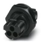
Circular connectors (device-side), Range of articles: PRC, Device connector, rear mounting, housing material: PPE, color: black, number of positions: 3, nom. voltage: 690 V AC, rated current: 35 A, Connection method: Crimp connection, Type of contact: Pin
