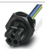
Circular connectors (device-side), Range of articles: PRC, Device connector, rear mounting, housing material: PPE, color: black, number of positions: 3, max. conductor cross section: 2.5 mm², nom. voltage: 690 V AC, rated current: 24 A, Connection method: Crimp connection, Type of contact: Pin, cable length: 150
