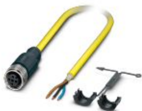
Sensor/actuator cable, 3-position, PVC, yellow, shielded, free cable end, on Socket straight M12, coding: A, cable length: 5 m
