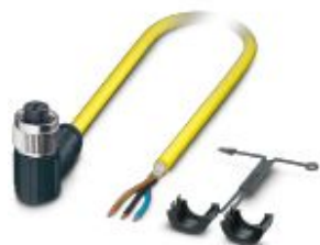
Sensor/actuator cable, 3-position, PVC, yellow, shielded, free cable end, on Socket angled M12, coding: A, cable length: 10 m
