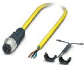
Sensor/actuator cable, 3-position, PVC, yellow, Plug straight M12 SPEEDCON, coding: A, on free cable end, cable length: 10 m
