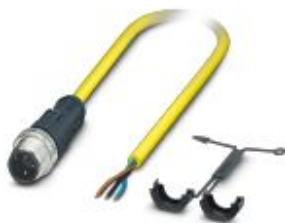
Sensor/actuator cable, 3-position, PVC, yellow, Plug straight M12 SPEEDCON, coding: A, on free cable end, cable length: 5 m
