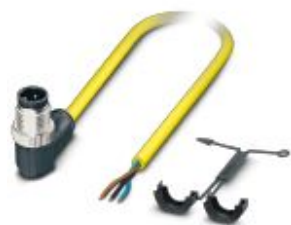
Sensor/actuator cable, 3-position, PVC, yellow, Plug angled M12 SPEEDCON, coding: A, on free cable end, cable length: 5 m
