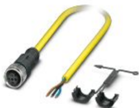
Sensor/actuator cable, 3-position, PVC, yellow, free cable end, on Socket straight M12 SPEEDCON, coding: A, cable length: 5 m
