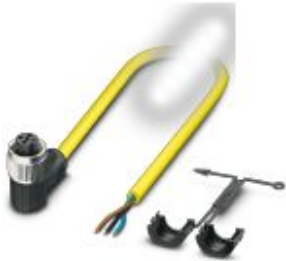
Sensor/actuator cable, 3-position, PVC, yellow, free cable end, on Socket angled M12 SPEEDCON, coding: A, cable length: 5 m
