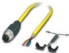
Sensor/actuator cable, 4-position, PVC, yellow, shielded, Plug straight M12, coding: A, on free cable end, cable length: 2 m
