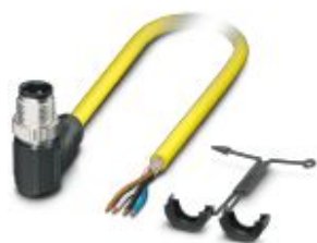
Sensor/actuator cable, 4-position, PVC, yellow, shielded, Plug angled M12, coding: A, on free cable end, cable length: 10 m
