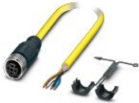
Sensor/actuator cable, 4-position, PVC, yellow, shielded, free cable end, on Socket straight M12, coding: A, cable length: 10 m
