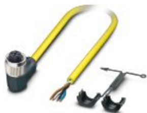
Sensor/actuator cable, 4-position, PVC, yellow, free cable end, on Socket angled M12 SPEEDCON, coding: A, cable length: 10 m
