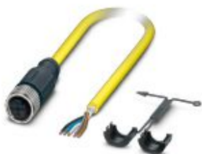
Sensor/actuator cable, 5-position, PVC, yellow, shielded, free cable end, on Socket straight M12, coding: A, cable length: 10 m
