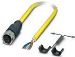
Sensor/actuator cable, 5-position, PVC, yellow, shielded, free cable end, on Socket straight M12, coding: A, cable length: 2 m
