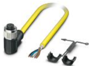
Sensor/actuator cable, 5-position, PVC, yellow, shielded, free cable end, on Socket angled M12, coding: A, cable length: 10 m
