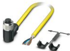
Sensor/actuator cable, 5-position, PVC, yellow, shielded, free cable end, on Socket angled M12, coding: A, cable length: 5 m
