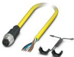
Sensor/actuator cable, 5-position, PVC, yellow, Plug straight M12, coding: A, on free cable end, cable length: 10 m
