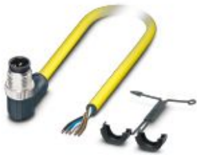
Sensor/actuator cable, 5-position, PVC, yellow, Plug angled M12, coding: A, on free cable end, cable length: 10 m
