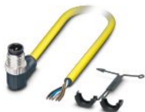
Sensor/actuator cable, 5-position, PVC, yellow, Plug angled M12, coding: A, on free cable end, cable length: 5 m
