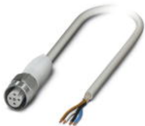
Sensor/actuator cable, 4-position, PP-EPDM halogen-free, gray RAL 7035, shielded, free cable end, on Socket straight M12, A-coded, cable length: 20 m, Hygienic design, with high-grade steel knurl
