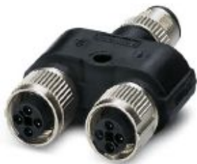
Y distributor, 4-position, Plug straight M12, coding: T, on Socket straight M12, coding: T and Socket straight M12, coding: T, For direct current up to 12 A/63 V
