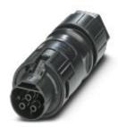
Circular connectors (cable-side), Range of articles: PRC, Coupler connector, type: Can only be released with a tool, housing material: PPE, color: black, number of positions: 3, min. conductor cross section: 1.5 mm², max. conductor cross section: 6 mm², nom. voltage: 690 V AC, rated current: 35 A, Connection method: Screw connection, Type of contact: Socket, min. cable diameter: 16 mm, max. cable diameter: 21 mm. Variant for release with a tool
