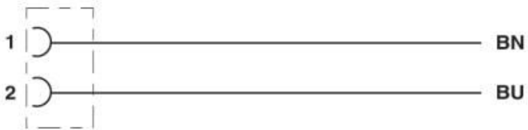
Contact assignment of the DEUTSCH DT06-2S
