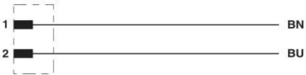
Contact assignment of the super seal plug
