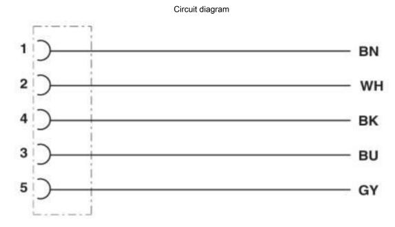
Contact assignment of the M12 socket
