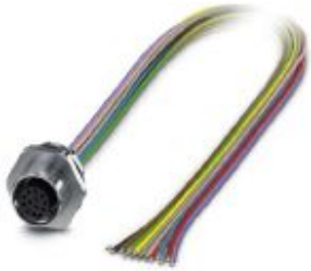
Flush-type connector, Universal, 12-position, Socket, M12, A-coded, Front mounting, M16 x 1.5, Individual wires, cable length: 0.5 m, 0.14 mm 2 , TPE litz wire
