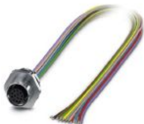
Flush-type connector, Universal, 17-position, Socket, M12, A-coded, Front mounting, M16 x 1.5, Individual wires, cable length: 0.5 m, 0.14 mm 2 , TPE litz wire
