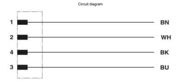
Contact assignment of the M12 connector
