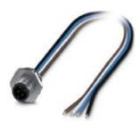
Flush-type connector, Universal, 4-position, Plug, M12, A-coded, Front mounting, M16  $\times$  1.5, Individual wires, cable length: 0.5 m, 0.34 mm², TPE litz wire
