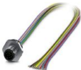
Flush-type connector, Universal, 17-position, Plug, M12, A-coded, Front mounting, M16 x 1.5, Individual wires, cable length: 0.5 m, 0.14 mm 2 , TPE litz wire
