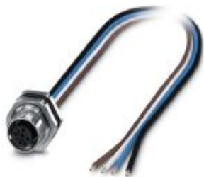
Flush-type connector, Universal, 4-position, Socket, M12, A-coded, Rear mounting, M16 x 1.5, Individual wires, cable length: 0.5 m, 0.34 mm², TPE litz wire
