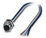
Flush-type connector, Universal, 5-position, Socket, M12, B-coded, Rear mounting, M16 x 1.5, Individual wires, cable length: 0.5 m, 0.34 mm<sup>2</sup>, TPE litz wire
