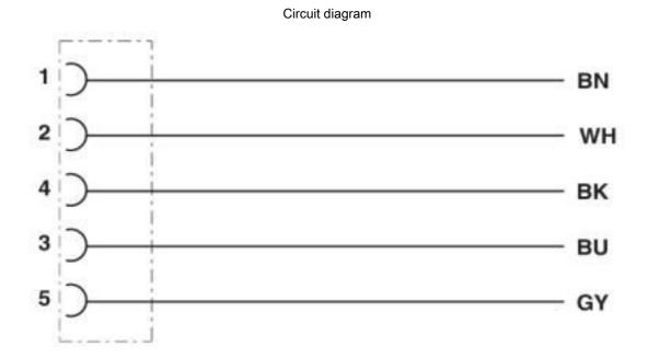
Contact assignment of the M12 socket
