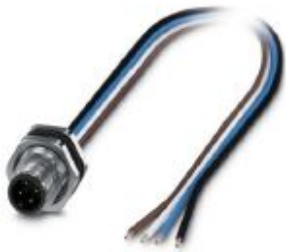
Flush-type connector, Universal, 4-position, Plug, M12, A-coded, Rear mounting, M16 x 1.5, Individual wires, cable length: 0.5 m, 0.34 mm 2 , TPE litz wire
