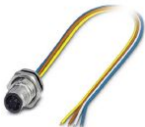
Bus system flush-type plug, PROFINET, 4-pos., M12 SPEEDCON, D-coded, rear/screw mounting with M16 thread, with 0.5 m TPE litz wire, 4 x 0.34 mm 2
