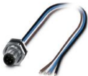
Flush-type connector, Universal, 5-position, Plug, M12, A-coded, Rear mounting, M16 x 1.5, Individual wires, cable length: 0.5 m, 0.34 mm 2 , TPE litz wire
