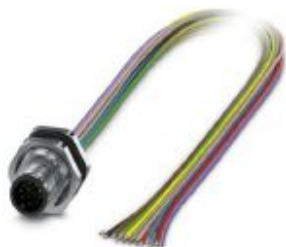
Flush-type connector, Universal, 17-position, Plug, M12, A-coded, Rear mounting, M16 x 1.5, Individual wires, cable length: 0.5 m, 0.14 mm 2 , TPE litz wire
